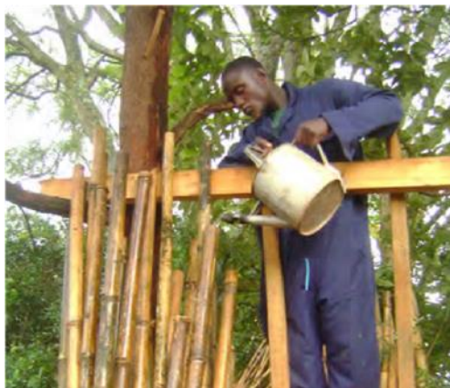
Figure 17: Addition of borax solution to standing culms
