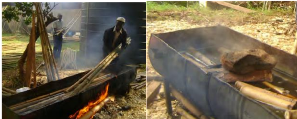
Figure 18: Heating bamboo in borax solution
